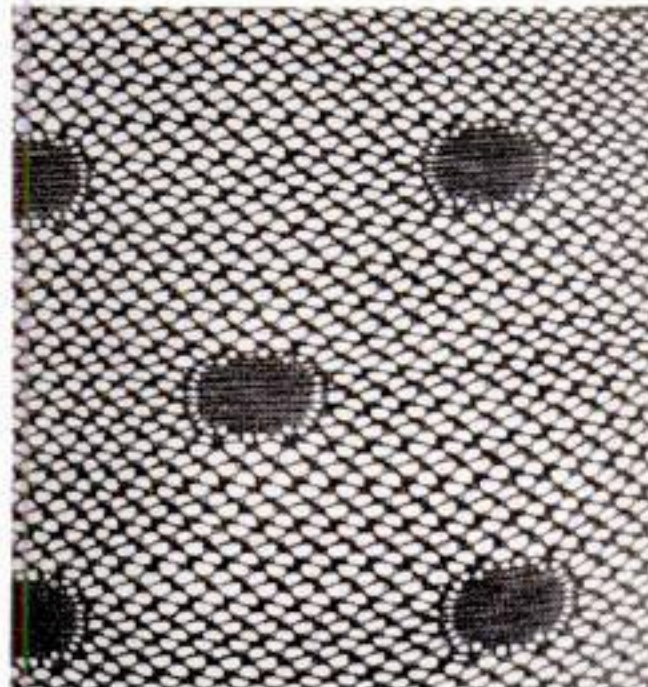
Coin-dot Lastex weave is used for girdle above. Weight: 1 1/6 oz., control 1/2 in.
